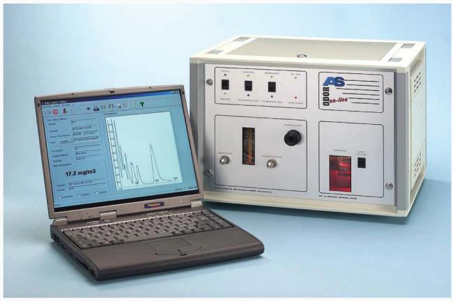
nline measuring: In gas networks of a suitable type of continuous, automatic measurement of the concentration of odorants is the safest, simplest method of maintaining an overview of odorant concentration in the network. In many cases, e.g. where the gas has alrady been odorized by the preivous supplier or the gas is odorized centrally at only a few stations, the automatic measuring technology ensures the greatest safety by enabling remote transmission, checks on the alarm etc.
